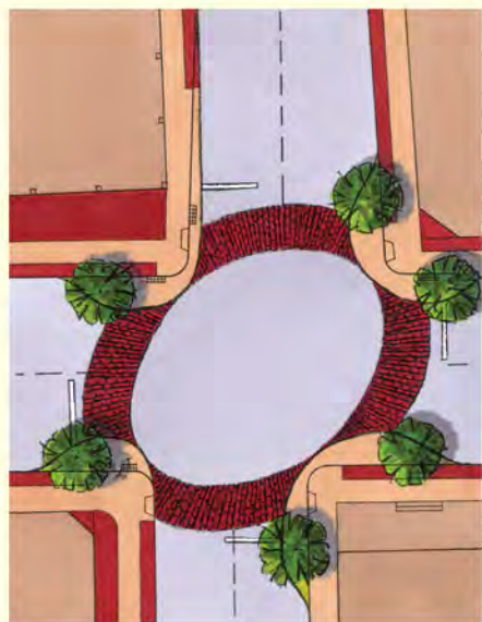
A redesign for the "four corners" intersection in Tivoli calls for textured brick crosswalks, street trees, and flared sidewalks out into the parking lanes to slow traffic, increase pedestrian visibility, and prevent illegal parking too close to the intersection.
