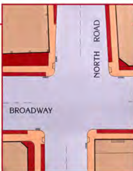
A redesign for the "four corners" intersection in Tivoli calls for textured brick crosswalks, street trees, and flared sidewalks out into the parking lanes to slow traffic, increase pedestrian visibility, and prevent illegal parking too close to the intersection.
